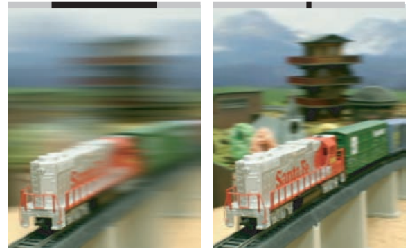
Figure 9: Simulated display views without depth compression (left) and with depth compression (right). We map the locomotive into the depth of field of the display, which reduces the maximum display disparity from 206 to 10 pixels.
