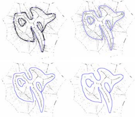
Figure 2: Medial axis filtering on a 2D shape (blue). The \lambda -medial axis is depicted in black. Top left: all extracted poles. Top right: pole filtering with parameter \lambda = 0.01 . Bottom left: \lambda = 0.03 . Bottom right: \lambda = 0.05 . To get a better sense of these parameters: the diagonal length of the bounding box of the input point set is 1.4.
