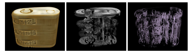
Figure 2: Volume visualisation integrated within the Wing device showing some of the API commands available and also illustrating the interactive 2D histogram transfer function manipulator with three results. In this example it clearly shows the internal pin mechanism for a dual-lock homeland securite padlock, highlighting, as well as the combination also defects in the metal casting.
