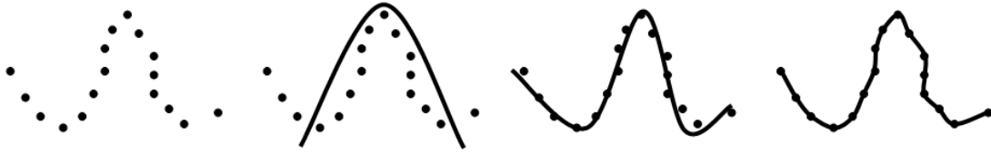
Figure 1: (a) A noisy point set. (b) An underfitted model. (c) A model with appropriate level of complexity. (d) An overfitted model.
