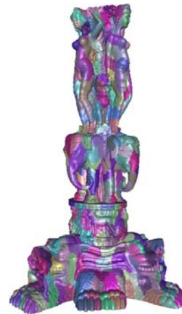
Figure 1: Mesh cutting result of the Thai Statue model. The resolution of the uniform grid is 512 \times 512 \times 512 ( n=8 ). The count of clusters is 512.
