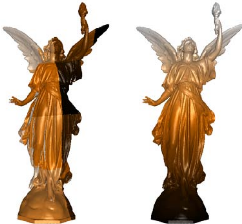
Figure 5: Mesh data locality optimization. Shading color displays the triangle sequence before (left) and after (right) the geometrical sorting.
