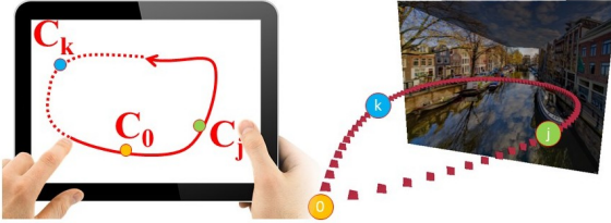
Figure 6: Stroke based animations. Various interactive and meaningful animation paths can be easily created by interpolating between few control points created with simple stroke inputs.
