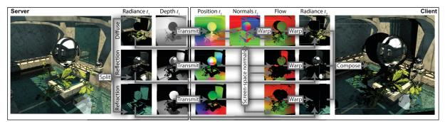
**Figure 2:** The server splits the rendering into a diffuse, a reflective and a refractive RGBZ image which are transmitted to the client. To create novel views, the client first decodes the diffuse positions and normals and subsequently the specular positions. These are used to create the flow to be applied to each node. Finally, the warped images are composed for the result image.
