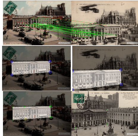
Figure 2: Façades identification (middle row) based on automatically matched features in the images (top row) and previously registered façade. Interactive selection of façade corners (bottom row). The example represent a partially visible façade case.
