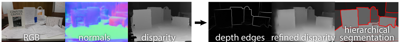
Figure 1: We present DEPTHCUT, a method to estimate depth edges with improved accuracy from unreliable input channels, namely: RGB images, normal estimates, and disparity estimates. Starting from a single image or pair of images, our method produces depth edges consisting of depth contours and creases, that separate regions of smoothly varying depth. Complementary information from the unreliable input channels are fused using a neural network trained on a dataset with known depth. The resulting depth edges can be used to refine a disparity estimate or to infer a hierarchical image segmentation.
