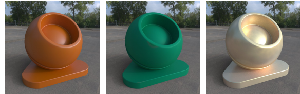
Figure 7: Three materials of the sample material set [Rus14] measured with the Radiant Zemax Imaging Sphere device: Basketball, green felt, and gold silver.
