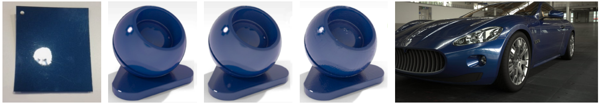
Figure 8: From left to right: a) A physical car-paint sample, b) its measurement, c) with an added clear coat (a Fresnel-layered specular BRDF), d) a normal map for scratches in the paint, and e) a rendering of the final material on a car model.
