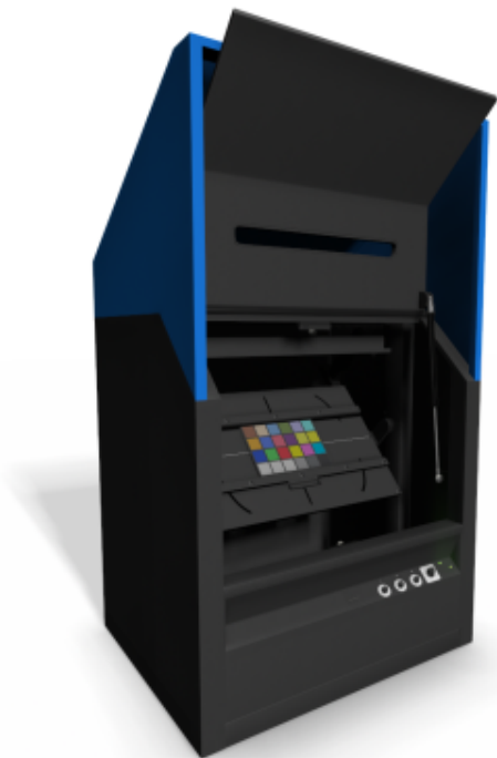
Figure 2: Simulation of a light booth with an adjustable easel. The light source direction remains constant with respect to the sample as the viewing angle changes.
