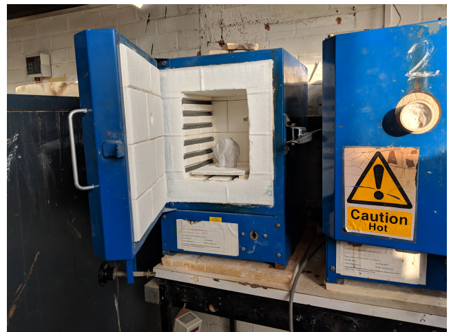
Figure 14: 3D printed elephant shape in the kiln ready for firing.
