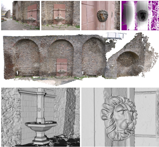
Figure 13: The Citywall dataset. The top row shows 3 out of 363 input images and one depth map. The middle row shows the full reconstruction in color, and the bottom row shows the fountain and a small detail on the fountain.
