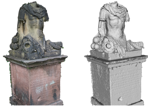
Figure 5: The final surface reconstruction with color (left) and shaded (right). Notice how even the engraved text is visible in the geometry.
