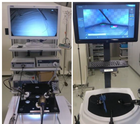
Figure 1: [left] typical box trainer versus [right] virtual reality trainer (LAP Mentor™, Simbionix)
