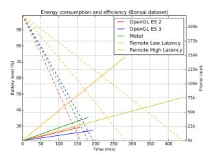
**Figure 2:** Energy consumption (dashed lines) and number of total rendered frames (solid lines) over time for a test run from a battery level of 100% down to 20% for a variety of different renderers on the iPhone 6 Plus with the highest quality settings.
