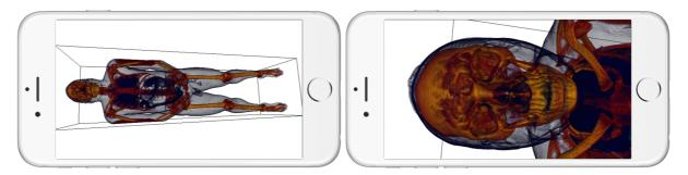
**Figure 1:** Next generation low-level graphics APIs allow for unprecedented performance on mobile devices. The Visible Human CT dataset with a resolution of  $256 \times 256 \times 942$  voxels ray-casted at interactive frame rates of 5 FPS (left) and up to 7 FPS (right).
