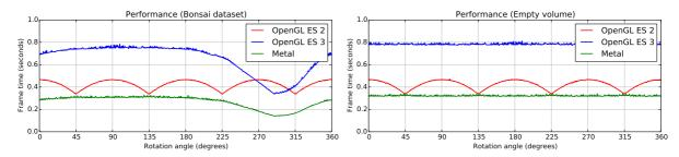
**Figure 3:** Frame times for the 360-degree rotations around the x-axis of the Bonsai dataset (left) and a volume with a totally transparent transfer function (right). The empty volume prevents early ray termination and thus forces many samples, which states the worst case scenario.
