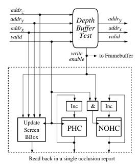
Figure 12: Schematical description of the Occlusion Unit.
