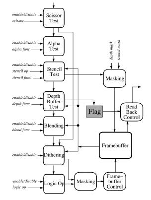
Figure 11: Schematic of the per-fragment-stage of the graphics pipeline illustrating where the occlusion flag is established.
