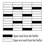
Figure 2: Progressive sampling of the virtual occlusion buffer using a sampling value of 6. Hence, after six sampling iterations, the correct occlusion information will be retrieved.
