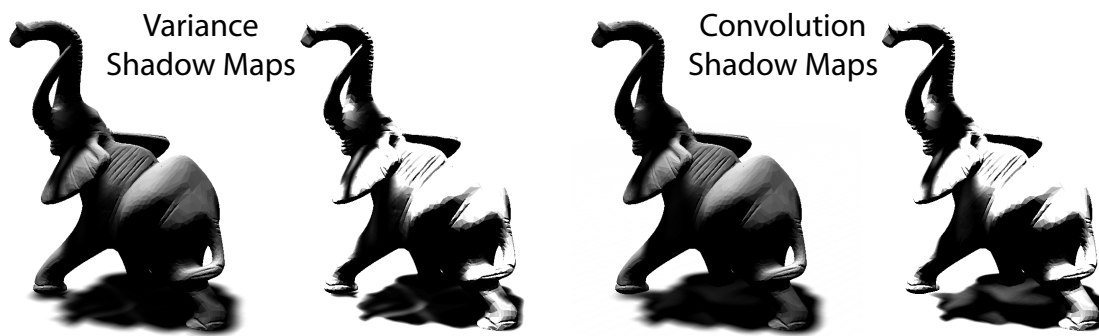
Figure 4.9 Although some light bleeding is present in approximate solutions (VSM: left, CSM: right, each original and scaled with a factor four), newer approaches show significantly less artifacts and are a good choice when high performance is needed.
