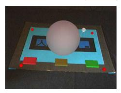
Figure 3: Buttons in the workspace to remove the need for keyboard input.
