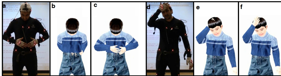
Retargetting for online performance animation on two postures. (a, d) Performed postures (b, e) Results of Kulpa et al. [1]. (c, f) Our results.
