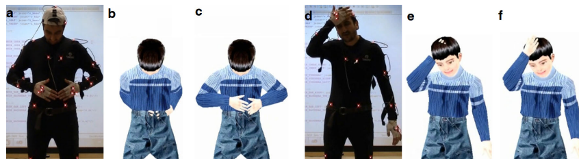
Figure 1: Retargetting for online performance animation. Variation in proportion and thickness between the performer and the avatar causes artifacts in case of self-body interactions. (a, d) Performed postures. (b, e) Resulting postures with [KMA05]’s technique. (c, f) Our results.
