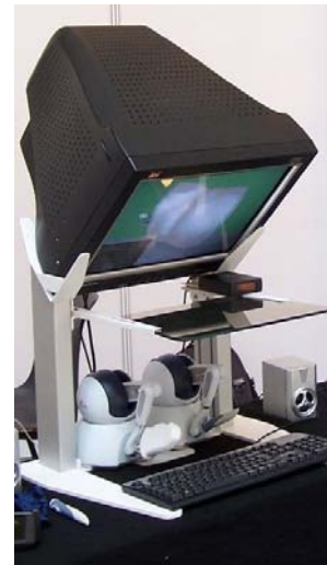
Figure 1: ImaGINE-S Platform: A virtual workbench with two PHANToM Omni haptic devices (one for the needle and one for the ultrasound transducer)
