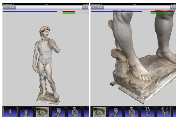
Figure 2: Precomputed view positions. The interface provides the possibility of browsing a list of pre-computed view positions (bottom side of the interface).
