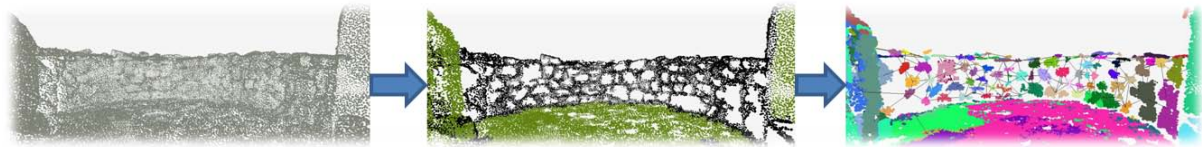
Figure 1: Automatic Point Cloud Segmentation Pipeline - Raw data is first segmented into smaller patches then geometric planes (coloured patches) are mapped onto these segments using the RanSaC paradigm
