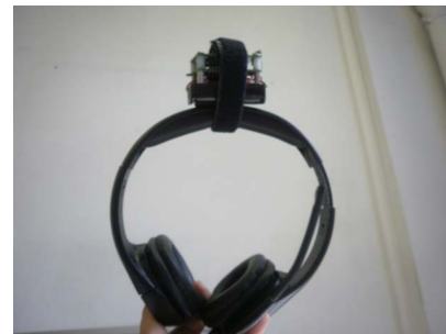
Figure 4: Orientation sensor fixed on headset.
