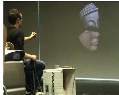
Figure 3: The bimanual tangible user interface
