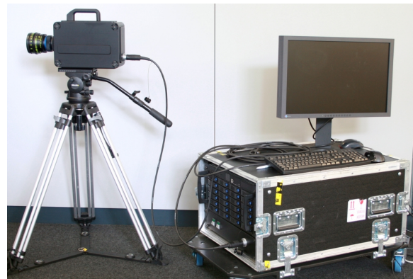
Figure 2: A photograph of the HDR video camera setup.
