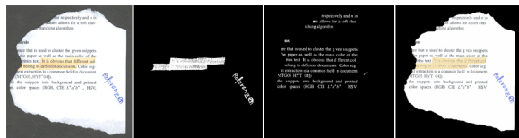
Figure 8: Segmentation result of a snippet: (a) original image, (b) segmented colors, (c) segmented black/gray and (d) final image colors
