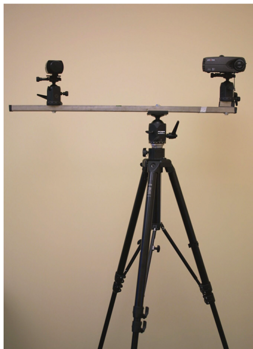
Figure 5: The re-configurable structured light scanning gantry consisted of a digital camera, a projector and a tri-pod mounting system.
