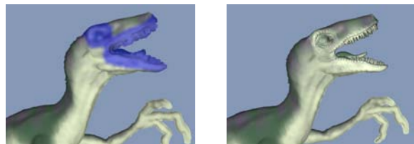
Figure 3: Multi-scale painting. Left: After having roughly painted on it, the user selects an area (in blue) of the low-res sampled object. Right: A local refinement is performed, by up-sampling the selected area from the original large model. Newly inserted samples are textured according the current PST defined by the in-core point set; the user can now paint smaller features.
