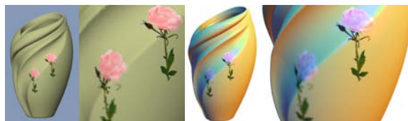
Figure 4: Topology-free painting with up-sampling. Left: The integration of bitmaps in the low resolution model (100k samples) can be done either by coloring existing surfels (left rose) or locally up-sampling the model to reach the brush resolution (right rose). Right: The high resolution mesh (7M polygons) textured with the edited point set. Note the difference in sharpness between the two roses, when the up-sampling is performed.
