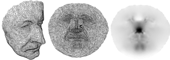
Figure 4: A surface triangulation \mathcal{M} and its parameter domain \omega . Distortion in the metric g is depicted by a density plot on the right, measured by Eq. (2) with a = \text{tr}(g^{-1}) , d = \det(g^{-1}) , \frac{\alpha_l}{\alpha_a} = 100 .
