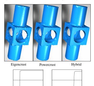
Figure 7: Reconstructions of a mechanical part by three algorithms. The eigencrust algorithm uses both eigenvectors, whereas the hybrid (spectral Powercrust) algorithm uses only the first.
