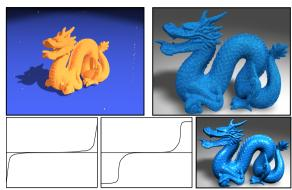
**Figure 8:** Eigencrust reconstruction of the Stanford Dragon model from raw data. The point cloud (upper left) has many outliers, which are automatically omitted from the spectrally recovered surface. 1,769,513 input points; 11,660,147 tetrahedra; 2,599,114 surface triangles; genus 1; 197 minutes reconstruction time.
