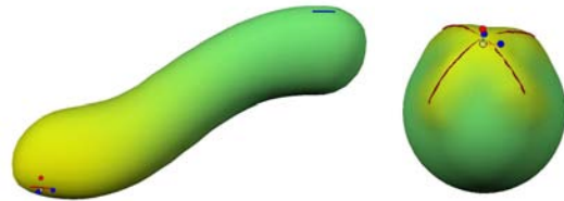
Figure 2: The designer can pull the model from several positions with multiple curves.
