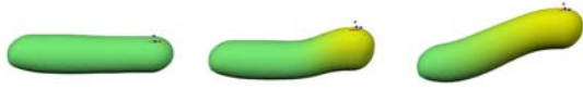
Figure 3: A peeling interface. Depending on how far the designer pulls the curve, the deformation region is determined.
