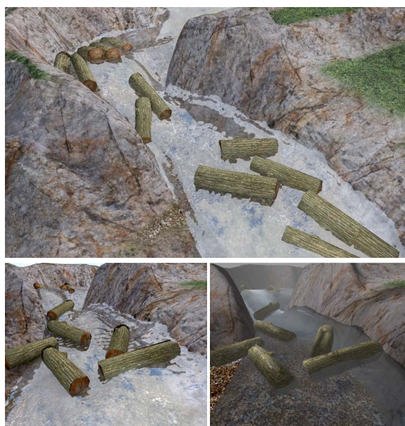
Figure 8: A dam built of several logs collapses, resulting in the fluid and the debris to flow down the valley. An unbounded domain is used, and the particles can flow to arbitrary locations. The bottom row shows different rendering techniques; on the left the surface is rendered offline with Povray, and on the right we used our real-time OpenGL renderer.
