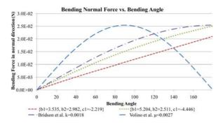
**Figure 10:** Bending force in normal direction for a single bending element using different bending models.
