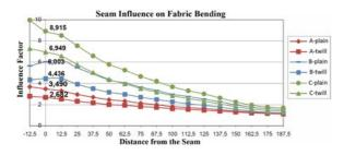
**Figure 5:** Influence of seams A, B and C on different types of fabrics, measured using the ACPM200. The influence factor describes the increase in stiffness in relation to the fabric without any seams.
