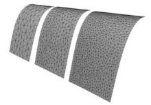
**Figure 3:** A stiff piece of cloth, simulated using three different mesh resolutions (150 faces, 574 faces, 1408 faces). The bending behaviour is virtually independent from resolution
