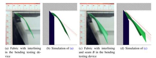
**Figure 7:** A comparison of results obtained using our bending and seam model with results using the bending stiffness tester ACPM200. The fabric sample (20cm wide) with interlining is simulated using bending coefficients { $b_1 = 0.5168$ ,  $b_2 = 1.8856$ ,  $c_1 = 2.2683$ } obtained from measurements. The seam is of type B, a safety-seam.
