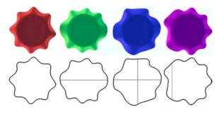
**Figure 8:** Drapemeter simulation. From left to right: no seam, a single seam along the weft direction, two seams aligned along weft and warp directions, and a seam that has been shifted to the side. The fabric bending stiffness parameters are  $\{b_1 = 0.1, b_2 = 0.0892, c_1 = -0.0092\}$ , the seam is simulated as a double lap seam.
