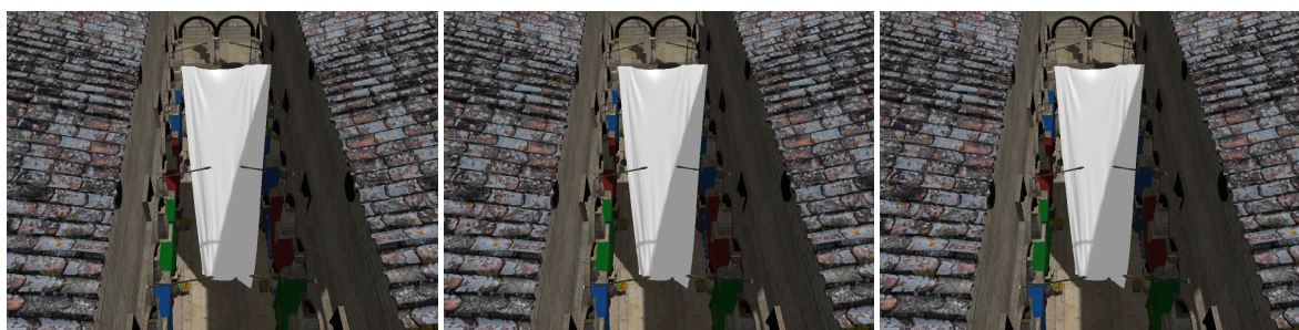
Figure 9: Visual Comparison using the complex Sponza Atrium scene: Left: Regular sampling with 289 shadow maps, acting as ground truth for our comparisons (2.5 FPS). Middle: Our method, 163 shadow maps (5 FPS). Right: Our method with only half the comparison render target size and a 3 \times 3 PCF filtering requires only 14 shadow maps and is rendered at 40 FPS. See Figure 10 for difference images.
