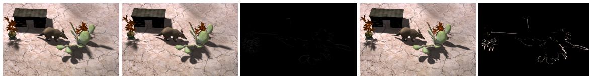
Figure 7: Visual Comparison, from left to right: (1) Regular sampling with 289 shadow maps, acting as ground truth for our comparisons (8 FPS). (2): Our method, 93 shadow maps (17 FPS). (3): Difference image between ground truth and our approach with 93 shadow maps, scaled by factor 5 for visualization purposes. (4) PCSS soft shadow solution with visibility calculated from only a single shadow map (64/64 samples for blocker search/filtering step, 370 FPS). (5) Difference image between ground truth and PCSS, scaled by factor 5 for visualization purposes.
