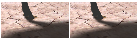
Figure 8: Left: Reducing the resolution of the comparison render target leads to the use of fewer shadow maps and therefore to banding artifacts. Right: By applying a simple 3 \times 3 PCF filter, the artifacts can be significantly reduced – but physical correctness is not guaranteed anymore.
