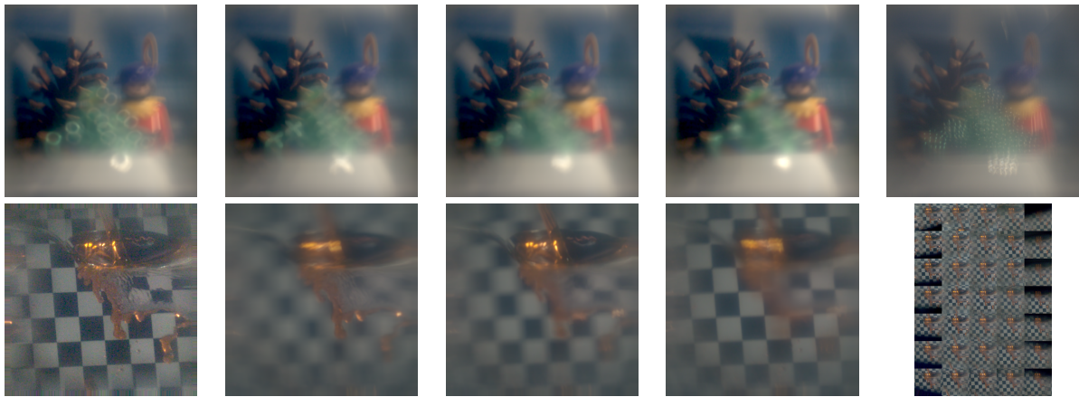
Figure 8: Refocusing results for light fields recorded with a faceted mirror setup after upsampling to 1617 images. The top row shows the result of simulating different aperture shapes for artistic bokeh control, the bottom row demonstrates refocusing for a short-exposure recording of liquid splashing off a spoon. The rightmost column shows refocusing using only the original 35 views (top) and the rectified input views (bottom). Please refer to the supplemental video for more examples.
