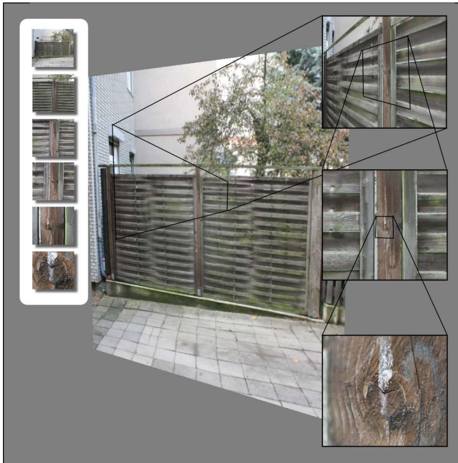
Figure 6: A zipmap texture acquired from six photographs and applied to a simple quad.
