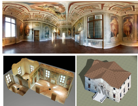
Figure 6: Some typical 3D modeling results from panoramic images based on interactive measurements.
