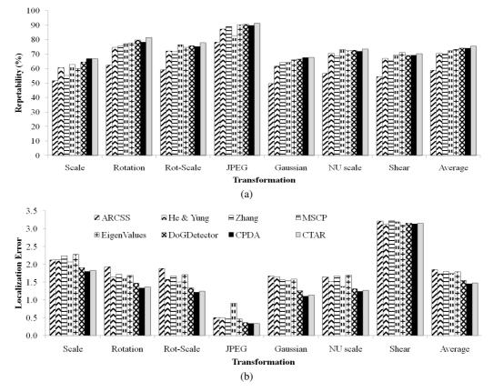
Figure 7: (a)Repeatability and (b)Localization Error by the corner detectors for different geometric transformation
