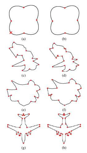
**Figure 6:** (a),(c),(e),(g) Corners detected by CPDA detector; (b),(d),(f),(h) Corners detected by CTAR detector
