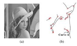
**Figure 2:** (a) Lena image; (b) Corners (denoted by 'o') detected by CPDA after removing weak corners.
