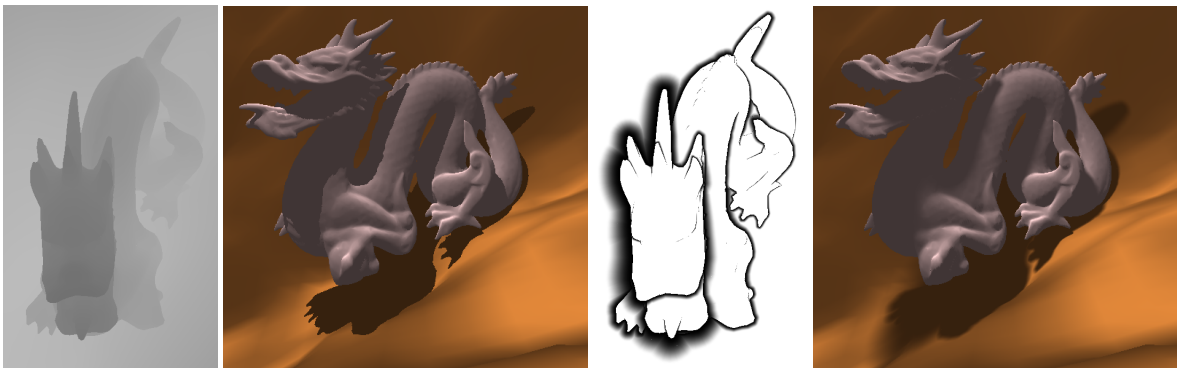
Figure 8: Using a standard shadow map results in hard shadows (left), add a penumbra map to get soft shadows (right). Using a 10k polygon dragon model for the shadows and a 50k polygon model to render, we get 14.5 fps at 1024x1024.
