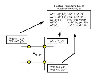
**Figure 5:** Floating-point jump map lookups. A vertex's texture coordinates are floating point, but jumps are only listed at integer addresses (circles) in the jump map. The jump lists (shown as "weight: <address>") from the neighbouring 4 integer addresses are concatenated, with bilinearly interpolated weights, and appropriately offset destinations, to form a jump list for a vertex's floating point address (top right).
