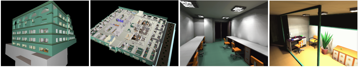
Figure 7: “Soda Hall”, a 7 storey fully furnished building containing 2.5 million triangles and 23,256 light sources. a.) The entire building, simply shaded, b.) Overview of a single floor c.) and d.) Inside, with full global illumination. With our proposed technique, the right images run at 2-3 frames per second on 22 CPUs allowing to interactively explore the entire building with full global illumination.
