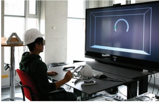
Figure 1: The experimental environment. The depth cues include the stereoscopic viewing, head tracking, head lighting, a 0.72\text{m} \times 0.4\text{m} \times 0.4\text{m} sized wire-frame box and a chess-board pattern floor.
