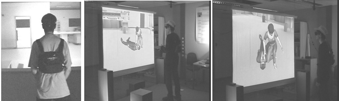
Figure 7 A trainee interacting with the system: hiding technology, stereoscopic immersion using rear projection and active stereo shutter glasses, natural voice interaction with the virtual assistant, intuitive navigation in virtual environment using wireless magnetic head tracking.
