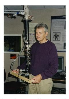
Figure 3: Argonne Arm with surrogate handles
