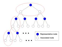
**Figure 2:** Only the nodes at every k levels starting from the root (drawn in blue) store the data blocks. The red ellipsis show examples of the distribution units. In the figure, k = 2 and h = 6. A binary tree rather than an octree tree is drawn here for illustration purpose only.
