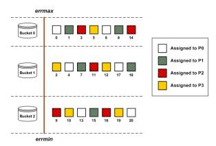
**Figure 4:** An example of data distribution along the hierarchical space-filling curve with error-guided bucketization. The numbers associated with the distribution units shown in the figure indicate the traversal order given by the spacefilling curve. In this example, a total of 21 distribution units with three different resolutions are distributed among four processors.
