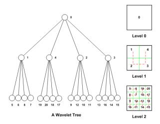
**Figure 3:** A simplified 2D example of data distribution along the hierarchical space-filling curve. All the wavelet tree nodes are traversed level by level in a breadth-first search manner. The numbers associated with the tree nodes indicate the traversal order given by the space-filling curve. A popular space-filling curve, the Hilbert curve, is used in this example.
