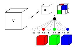
**Figure 1:** Calculating the error metric of a wavelet tree node *S*. *B* is the low resolution data block associated with *S*, representing the raw data subvolume *V*. The three colored nodes and their associated data blocks are examples used to illustrate the data relationship of the parent node *S* and it child nodes  $S_i$ , where  $0 \le i \le 7$ .
