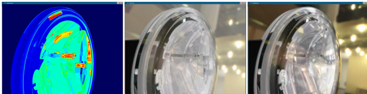
Figure 9: Number of rays used to compute each pixel (accuracy 95%). Each color represents a different number: black( < 1 rays per pixel), blue( \leq 10 ), magenta( \leq 20 ), green( \leq 30 ), yellow( \leq 40 ), red( > 50 ). The second and third images illustrate enhanced visual quality using a High Dynamic Range Environment Map: low dynamic range (second image), high dynamic range (third image).
