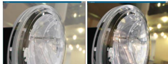
Figure 4: Enhanced visual quality using a High Dynamic Range Environment Map: Low dynamic range rgb environment map on the left, and a high dynamic range environment map on the right (see Figure 9 for a color version).
