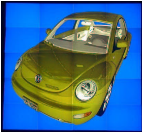
Figure 4: VW Beetle on a tiled screen driven by a cluster (Model courtesy Volkswagen, Image taken at NCSA using their Display Wall-In-A-Box implementation)
