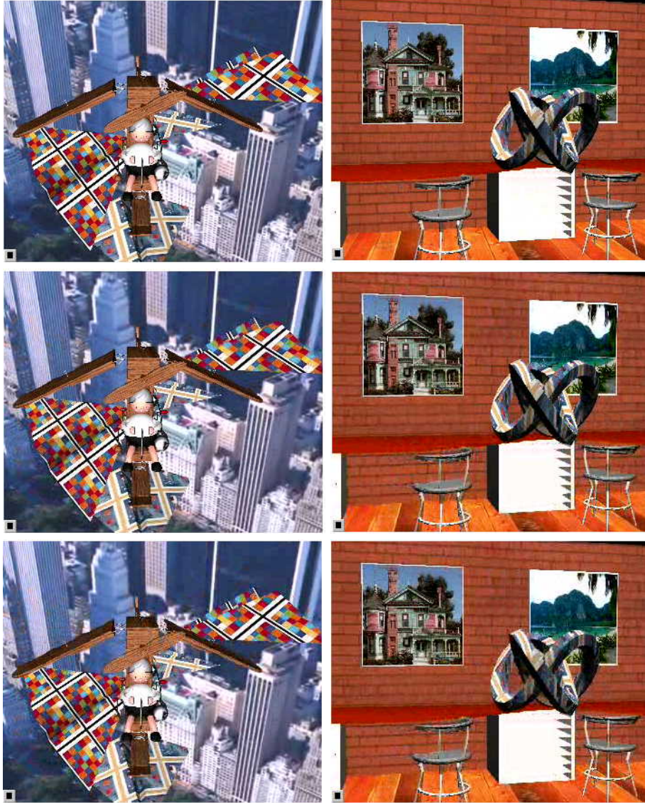
Fig. 4. A comparison of images encoded by our technique and naive quantization. In the upper row, the lowest value is used as the constant quantization value. While in the lowest row, the higher value is used. The middle row shows frames of our two-layer technique.
