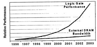
Figure 1: On chip vs. External Bandwidth
